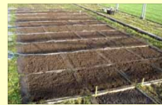
32 Lysimeters (1 x 1 x 1.5 m size)
